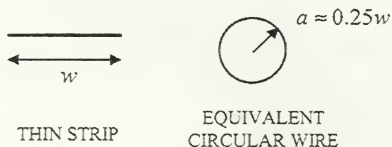
Figure 16: Equivalent thin strips and wires that is valid at low frequencies w < 0.1\lambda
